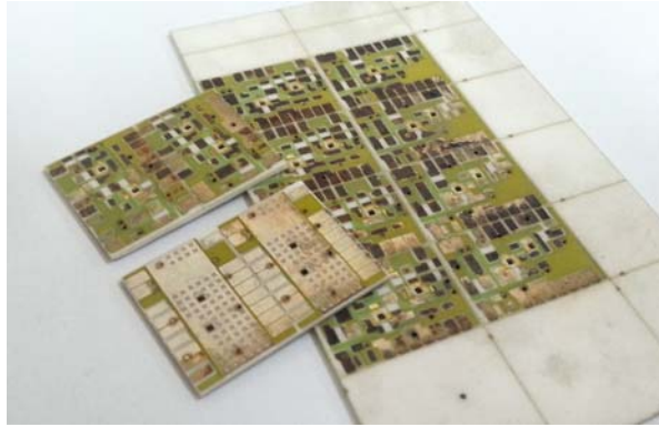
Figure 1.5 A photograph of substrates fabricated by thick film process
