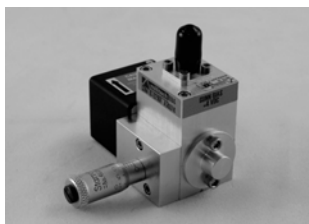
FIGURE 11.16 A W-band Gunn diode oscillator. The output power is 16 dBm, and the source is mechanically tunable over a frequency range of 4 GHz.
