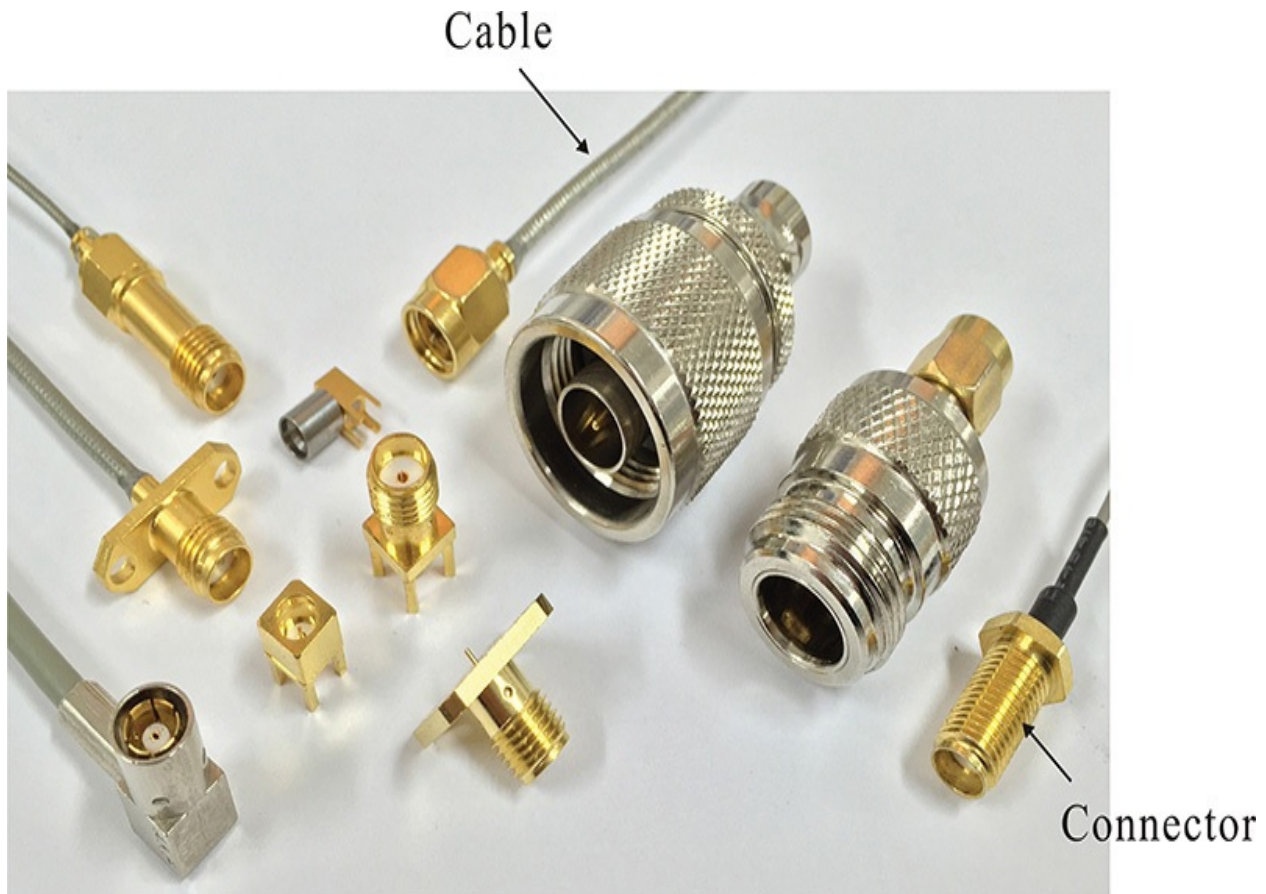
Figure 3.9 Photograph of various coaxial lines and connectors
