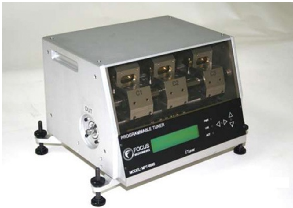
Figure 9.11 Photograph of an impedance tuner with three carriages. The three harmonic impedances can be separately controlled using this impedance tuner. Source: Focus Microwaves Inc., Three Carriage Three Harmonic Tuner, January 2012.
