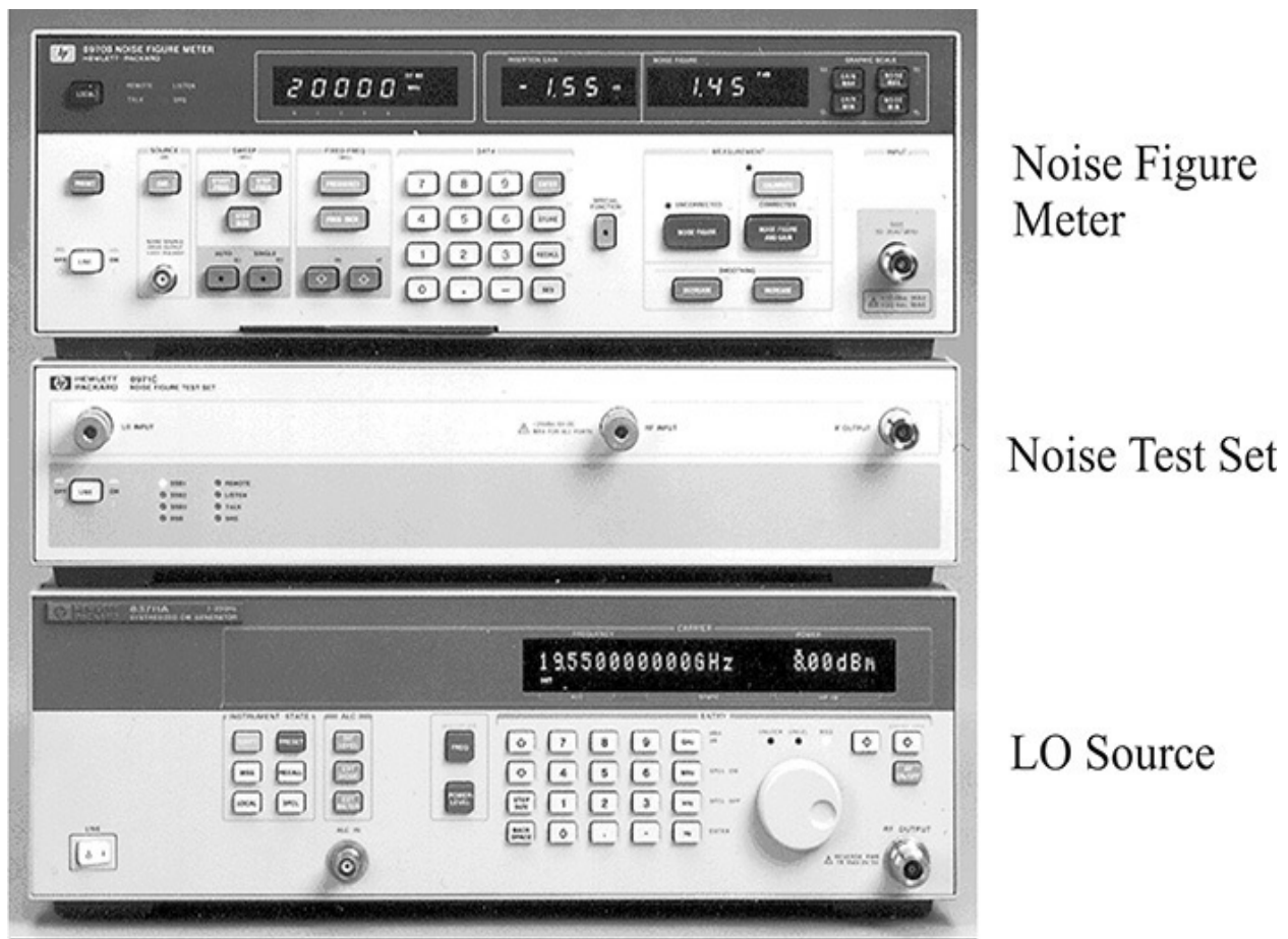
Figure 4.23 Noise figure measurement system. 3 The noise figure meter measures the noise figure of a DUT, but its frequency range is limited to 1.5 GHz. The noise test set is the down-converter for the noise figure meter. In the down conversion, an LO source is necessary. The signal generator at the bottom acts as the LO source for the down-conversion.
