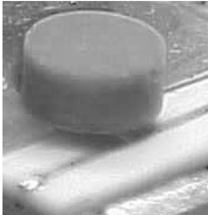
Figure 4-22 Dielectric resonator coupled to microstrip transmission line
